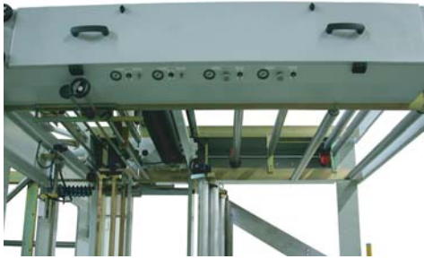
Double feed system driven by independent digital servo drives, fully programmable for synchronizing two printed reels.
