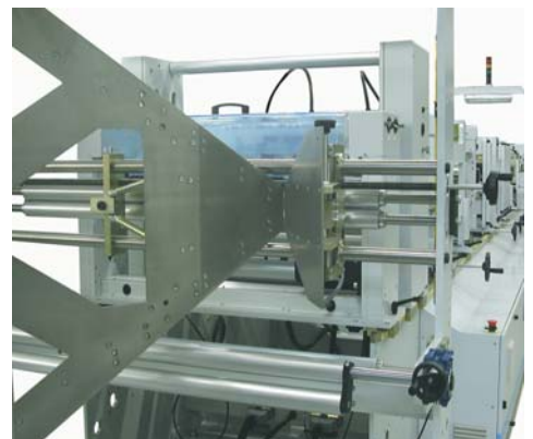
Folding station with gusset folding board. Replaceable folding board insert for gusset depth up to 150mm.
