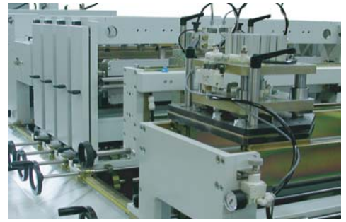
Cross sealing and cooling stations, driven by independent digital servo drives, fully programmable.
